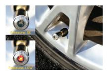
Once your fleet is equipped with the LED Smart Cap TPMS system, all your drivers need to do is walk around their vehicle and instantly know if a tire is low on pressure. No more fumbling around with tire gauges, tire bats, or worse complete neglect because checking tire pressures is too time consuming and difficult. This means that your fleet's tires can be properly inflated and you can be sure that your drivers are not telling you a lot of "hot air" when they say they checked their tires.
